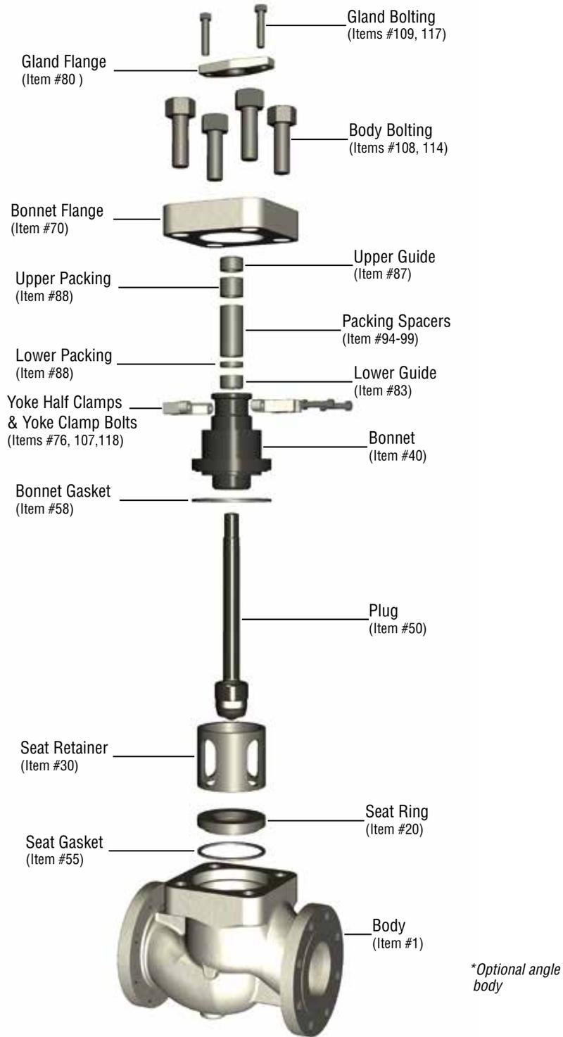
*Figure 3: Exploded View Mark One Body Assembly*
